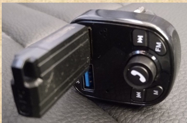
FM Transmitter and 16 Gig flash drive that plugs into the cigarette lighter socket
